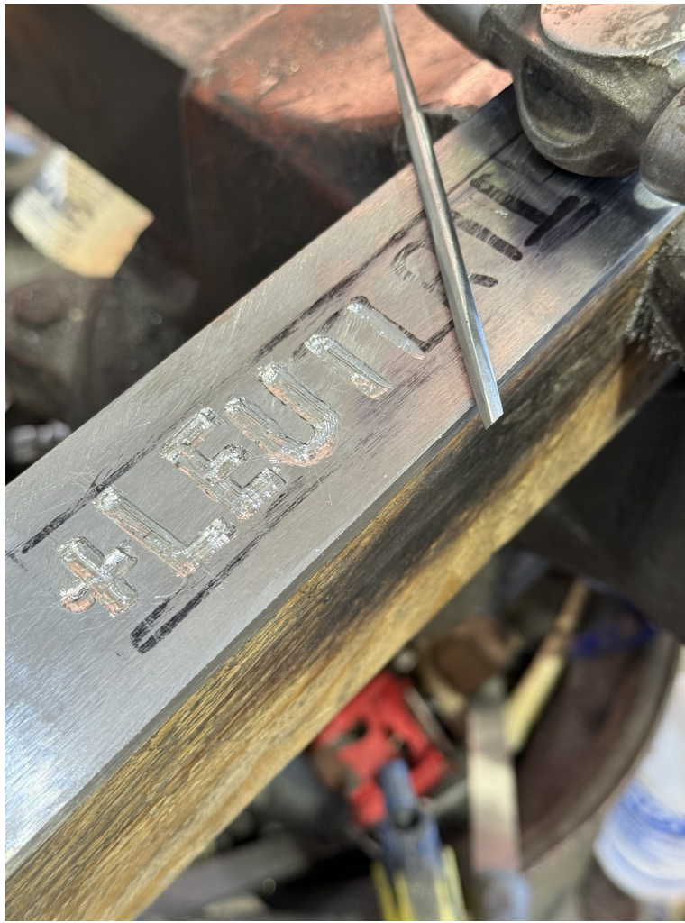
Figure 6. A closer view of the inlay work before final blade finishing. The modern example illustrates the practical steps, not a proven Viking Age procedure. Photograph: Atilivs Ironworks.
