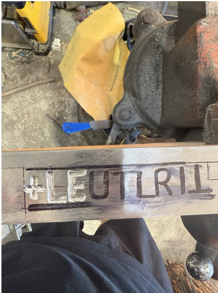
Figure 5. Inscription layout and early inlay work on the author's River Witham-inspired sword. Some strokes are already worked into the blade; the rest are marked for fitting. Photograph: Atilivs Ironworks.
